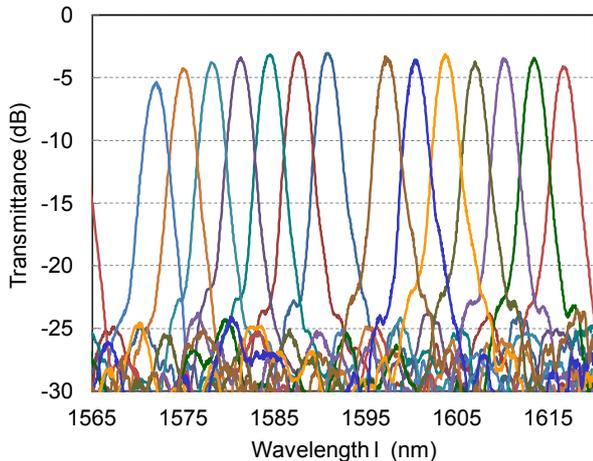
Fig. 2. Measurement result of 14ch-400GHz Si reflection-type AWG.
