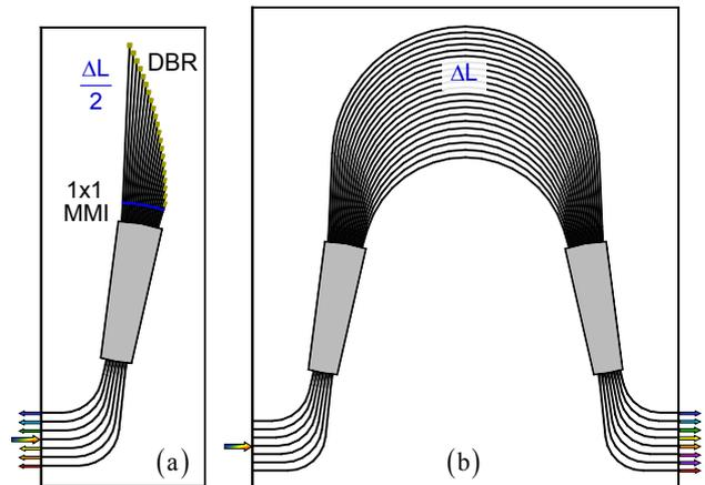
Fig. 1. (a) Reflection-type and (b) transmission-type AWGs.
