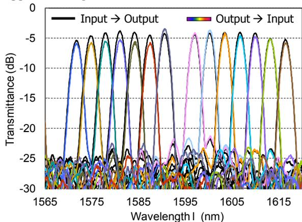
Fig. 3. Transmission spectra for the center input (black lines) and off-centered (colored lines) light coupling.
